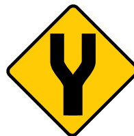
Yellow diamond 'Y' sign (road divides ahead)
